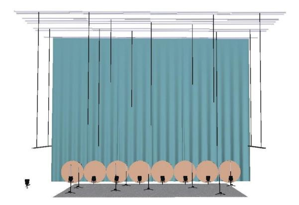
The lighting design for Out of Chaos contains 8 ropes (dyneema droppers) attached to fly bars which hang to specific heights above the stage. Each one has a magnet connection on the end of it. The performers attach and detach wireless Astera AX3 handheld LED lights to these magnet connections at different parts of the show. There is also one wireless Astera AX10 light attached to the most central rope for a scene in the show.
